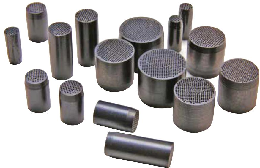
KIC Sintered Vents are composed of several straight and uniform pores made through a unique process to allow air or gas that gets trapped inside the mold cavity during the injection or die casting process to escape freely. To optimize mold design and reduce the possibility of manufacturing defective parts, specify strategically placed insertion points to hold the vents.
